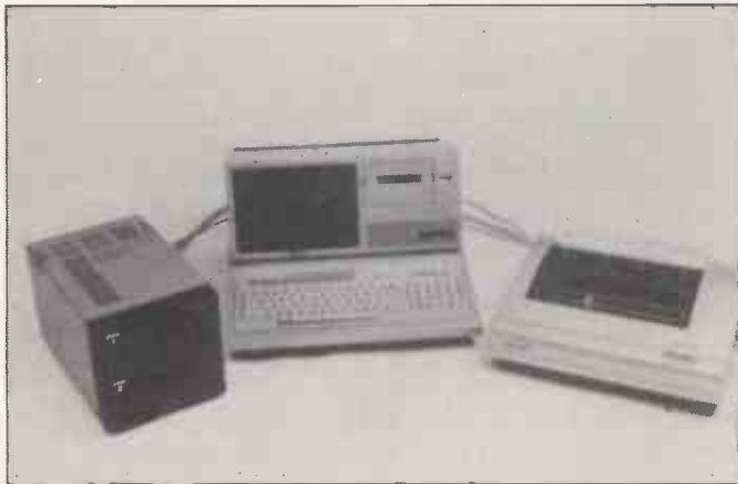
The Sharp MZ-80B is the follow-up to the popular MZ-80K and its main improvement over its precursor is the inclusion of the interface unit within the body of the main unit. High-resolution graphics and fast search on tape are other features of this machine. □
