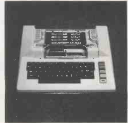
Atari 800 Console (with cover removed)
